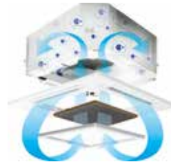
Ventilator circuleert nanoe™ X in de unit
